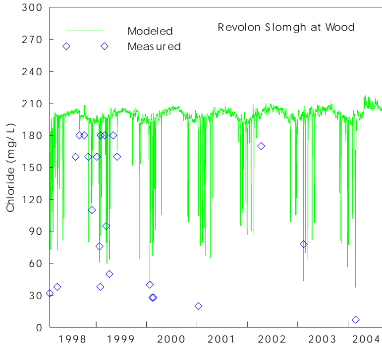
Figure 178: Measured and Modeled Chloride Time Series for Revolon Slough at Wood.
